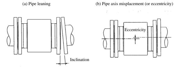
Figure 4.1 Pipe leaning and axis misplacement
